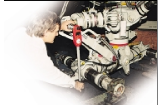
This CDS wrench is being used on the Landing Gear of a Boeing 747 aircraft.
